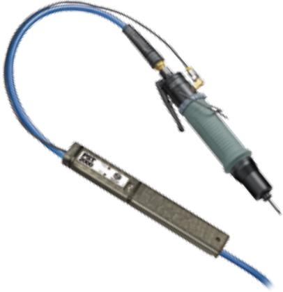
The PST 2000 works with ported auto-shutoff tools to create a profile of the air pressure over time during rundown and shutoff. The profile for a known conforming rundown and tightening is stored on the PST 2000, and all subsequent uses are compared to the profile. Conforming tightenings result in immediate feedback to the operator via an LED display, transmission to the Global Process Monitor, and confirmation on the display and LED's on the Process Monitor unit.
